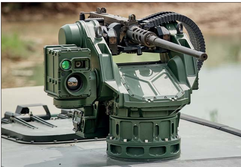
■ GLADIUS 12 RCWS is a modular concept, which allows the integration of 7.62 – 12.7mm machine guns and 30 – 40mm automatic grenade launchers
