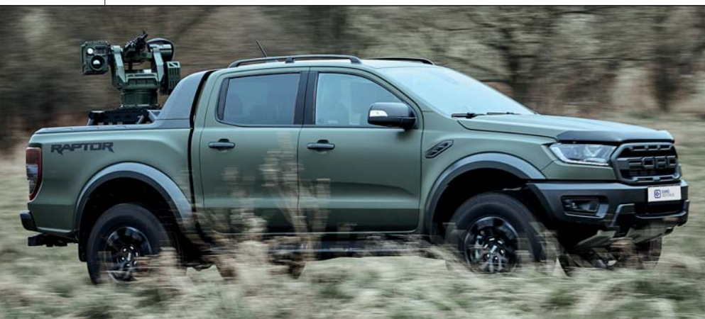
■ GLADIUS MINI RCWS with a 7.62mm machine gun on the Ford F-150 Raptor
